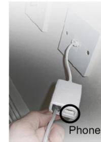
**1)** Plug a microfilter into your telephone socket. If you had to unplug something, you can plug it back into the "Phone" socket of the microfilter. It's best to leave it out until you've got everything working though.
